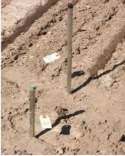
Gas Concentrations Measured with GasTek Model GV-100 Vacuum Pump *using either* No. 132 HA (1,3-D) No. 136H (MBr) Detector Tubes
