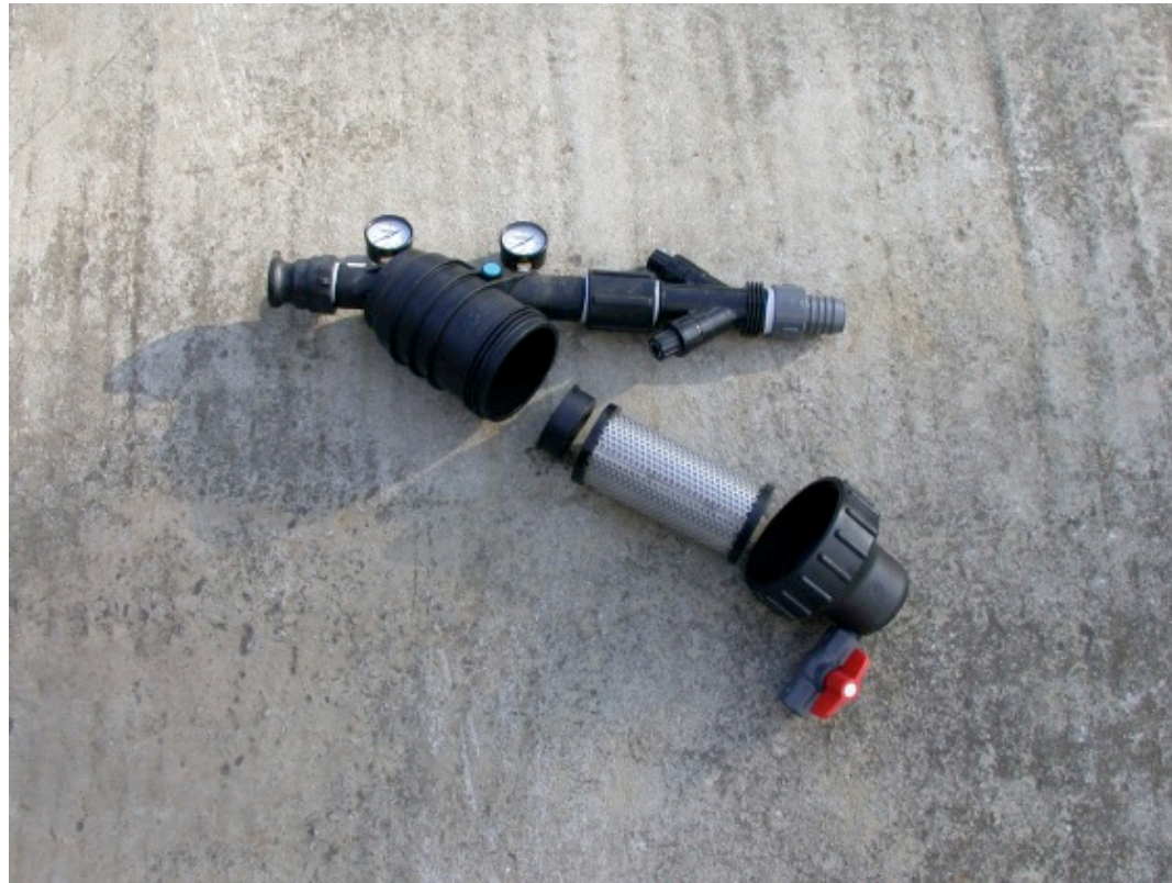
Figure 10. Disassembled screen filter with an incremental adjustable regulator
