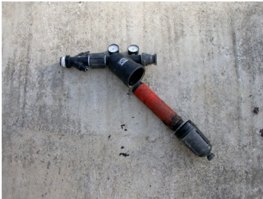
Figure 11. Disassembled disk filter with an incremental adjustable regulator
