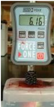
Figure 3. Wagner FDX force 1 gauge with 5 lb weight cell to measure of blackberries and raspberries.
