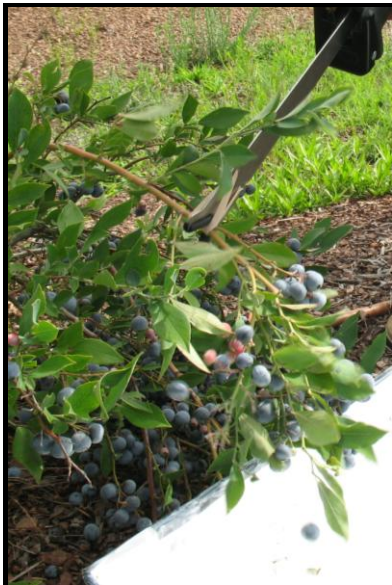
Figure 1: Mechanical shaker for fruit removal in blueberry. A reciprocating saw was modified by attaching a clamp and by addition of a resistor to enable fruit removal in blueberry.
