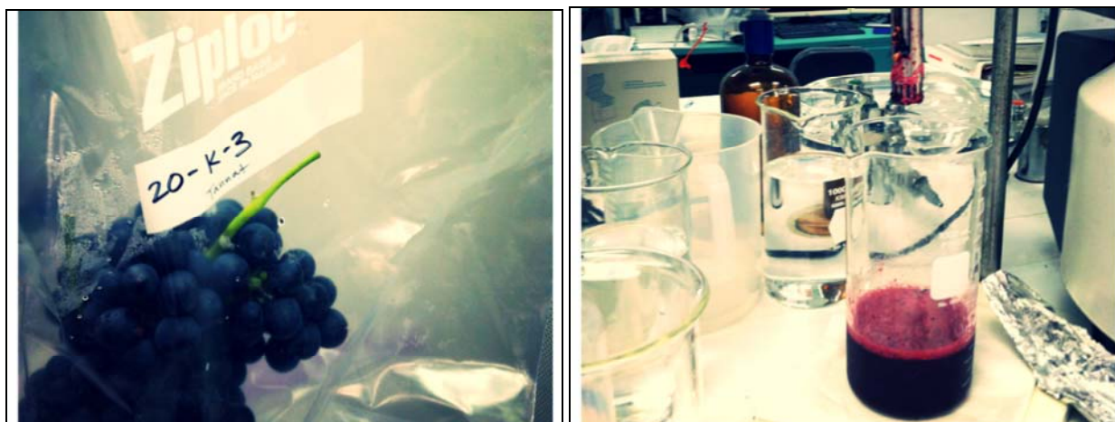
Figure 7. One wine grape sample (left). Two Tannat bunches in a Ziploc bag from Vineyard #20, sample #3. Polytron homogenizer creates grape must in a sterilized beaker (right).
