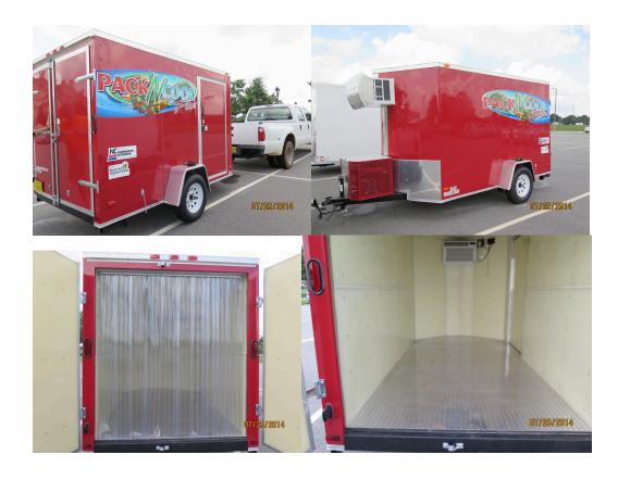
Figure 1. Pack N Cool Plus showing overall (A), front part with AC unit and baffle protector (top) and custom generator cage and generator (bottom) (B); curtain in back of trailer (C) and interior of trailer showing plastic sheeting, AC and cool bot, and diamond plate floor (D).
