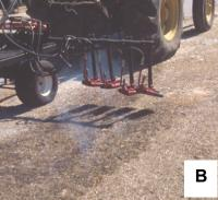
Fig. 1. Modified flame cultivator unit evaluated for suppression of mummy berry disease. Overall view of the unit (A); close-up view of a test run on a grassy surface (B); operation of the unit in a blueberry planting (C).
