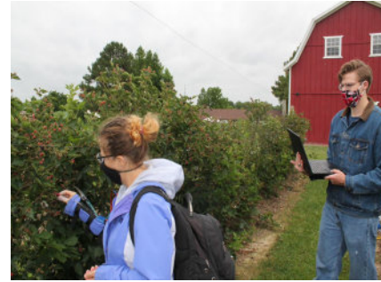
Fig. 2. University of Arkansas graduate students recorded and processed data for the force-sensing apparatus for fresh-market blackberry harvesting using a portable water-resistant case housed in a backpack. The resulting processed data was transmitted and logged to a mobile work-station.
