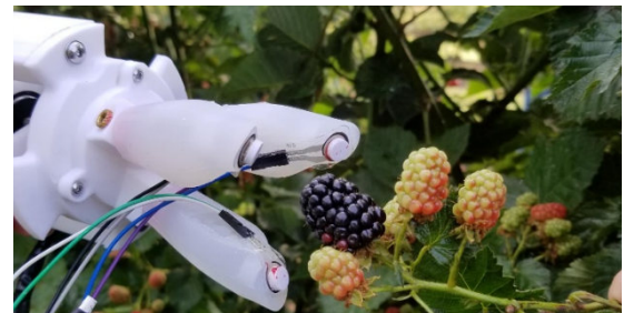
Fig. 3. Prototype of tendon-driven soft robotic gripper with compliant, soft material and active force feedback control for harvesting fresh-market blackberries.
