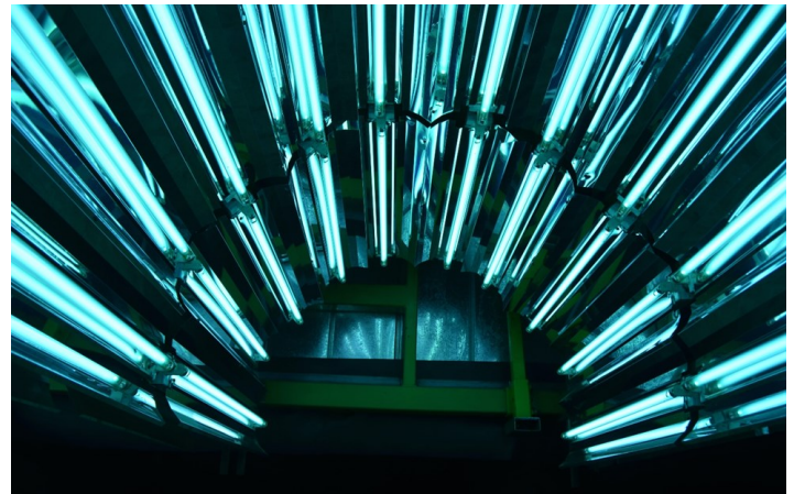
Fig 1. Interior of a reflectorized hemicylindrical array of germicidal UV-C lamps.
