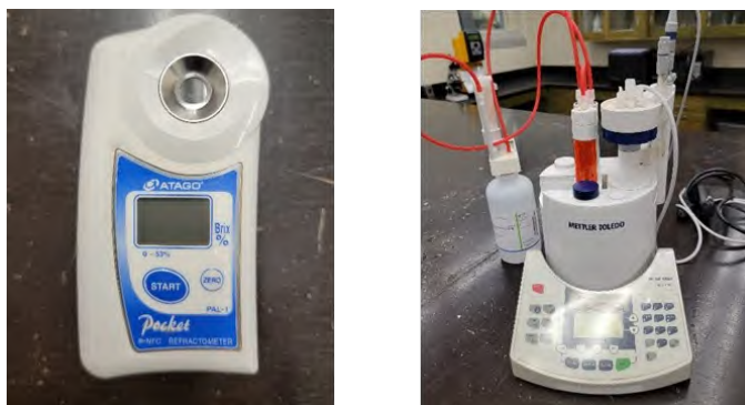
Figure 3. Postharvest equipment such as the hand-held Brix meter (A) or automatic titrator (B) which measures titratable acidity is important for quality data collection on small fruits.
