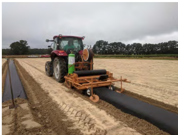
Figure 1-10. A single-row tractor towing a plastic mulch bed shaper with fumigation rig. Beds are pre-bedded through a single pass without plastic and fumigant application, and then followed up by a second pass, during which fumigants are applied and plastic is laid.
