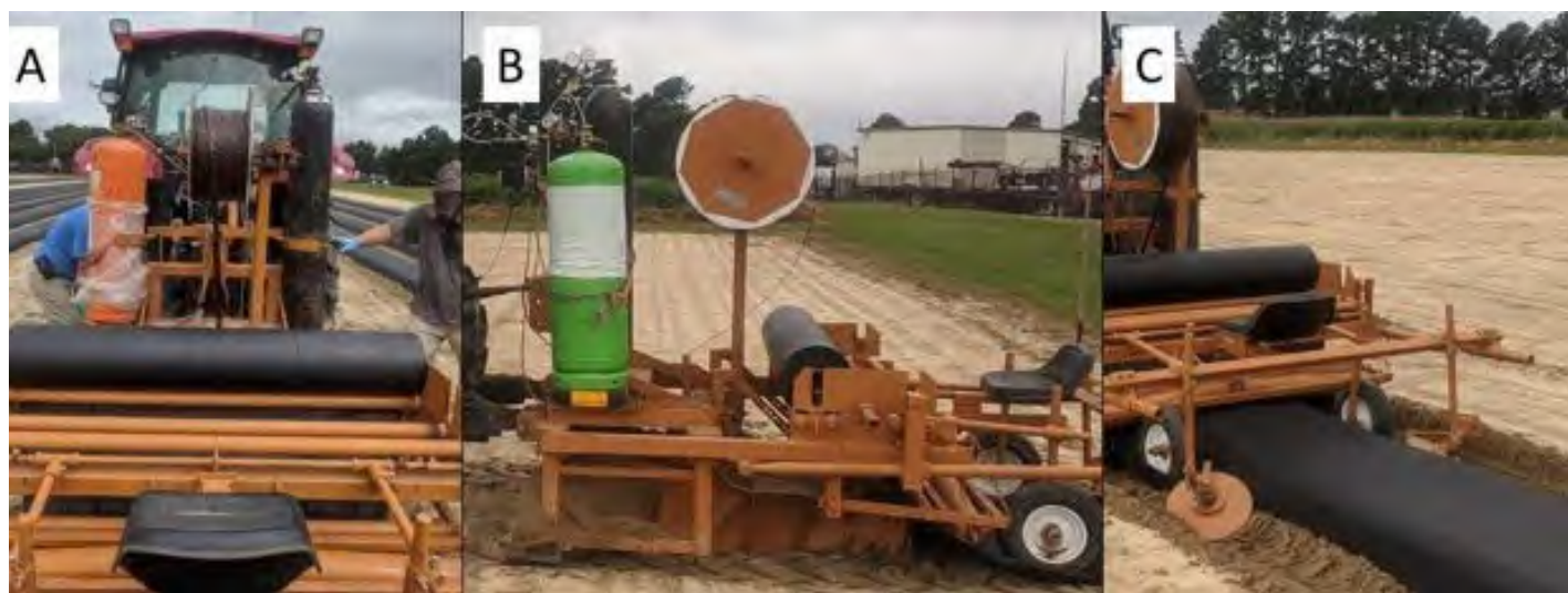
Figure 3-3. The fumigant tank, nitrogen gas tank, drip tape roll, and plastic mulch roll are visible on the fumigation rigs above. Beds should be pre-formed (first tractor pass) prior to application of the plastic, drip tape, and fumigant (second tractor pass). Multiple-row bed rigs are also available for larger farms.
